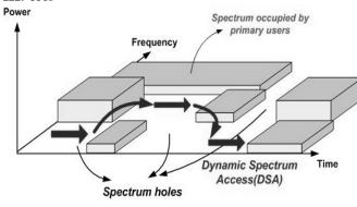
Fig. 2 Spectrum hole concept
